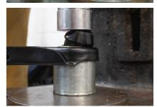
Figure 3. Bush pressed at an angle.
